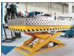
Ensuring safe standing or determination of optimum work height – wire encoders are used for support adjustment and control of elevating platforms.
