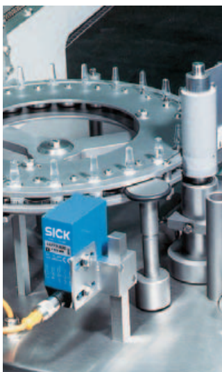
▲ Using luminescence scanners to detect presence of labels in the pharmaceutical industry.
