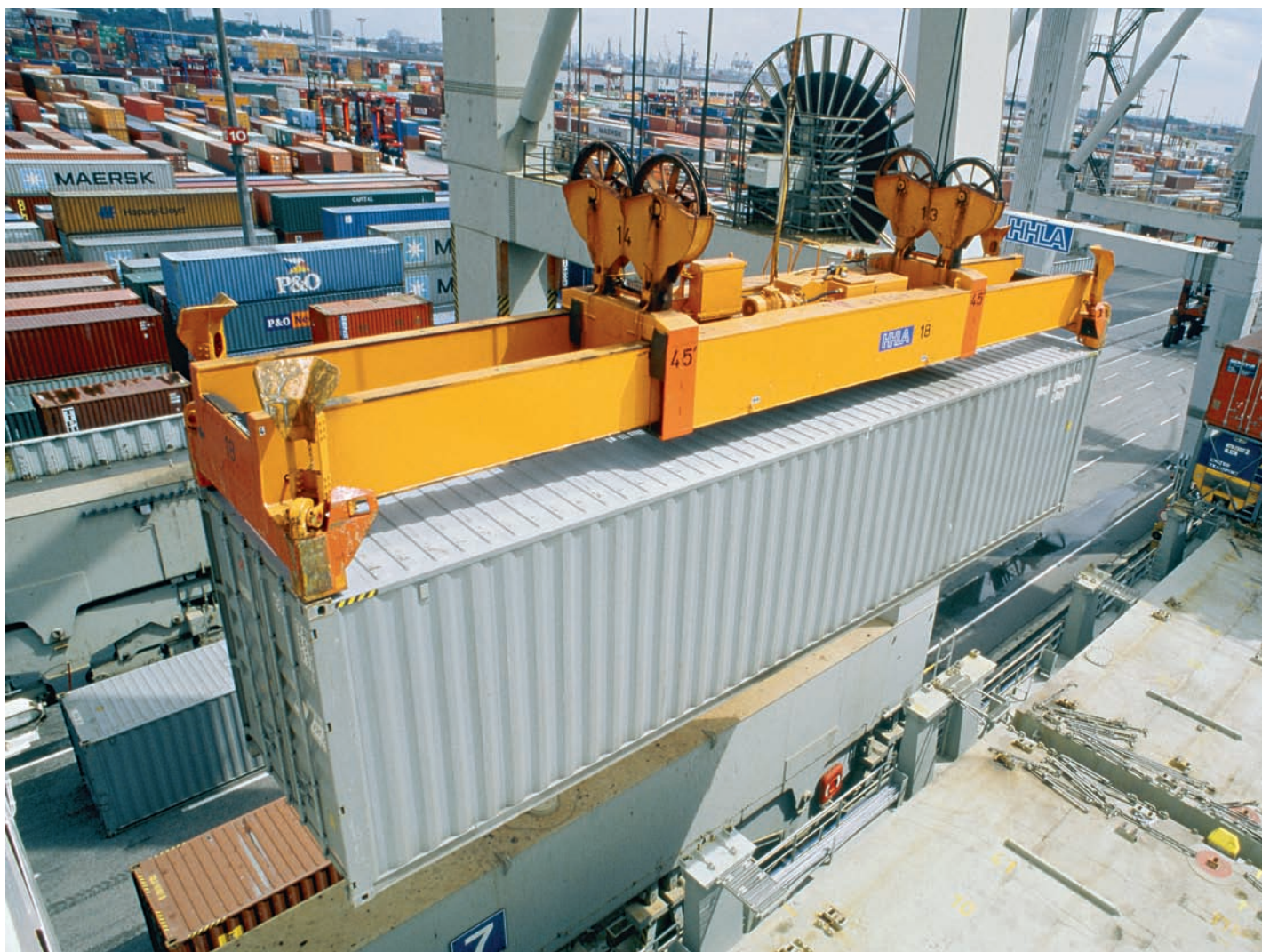
▲ The human eye is incapable of crane positioning in external applications. Exact distance measurement using the distance measuring devices DMT and DML ensures the necessary accuracy is achieved.
