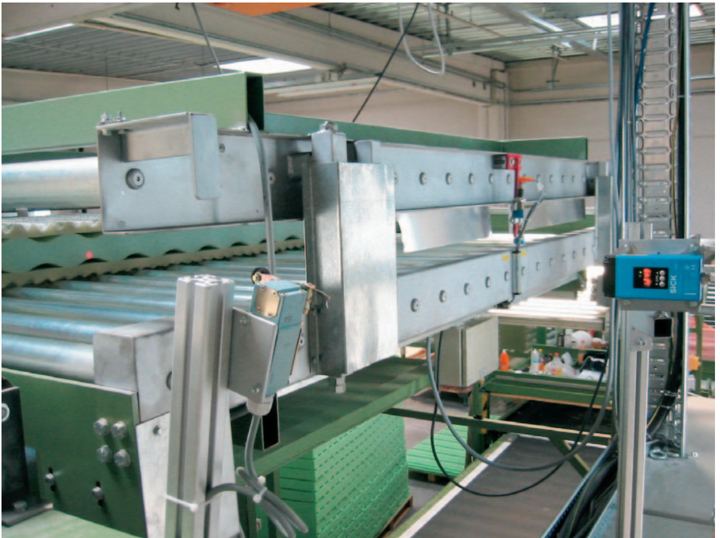
▲ A DT 500 laser sensor ensures the central positioning of mattresses and prepares them for bonding on the top layer of the mattress.
