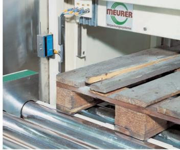
▲ With its eight parallel light beams, the WLG 12 reflex light grid can detect any damaged pallets.
