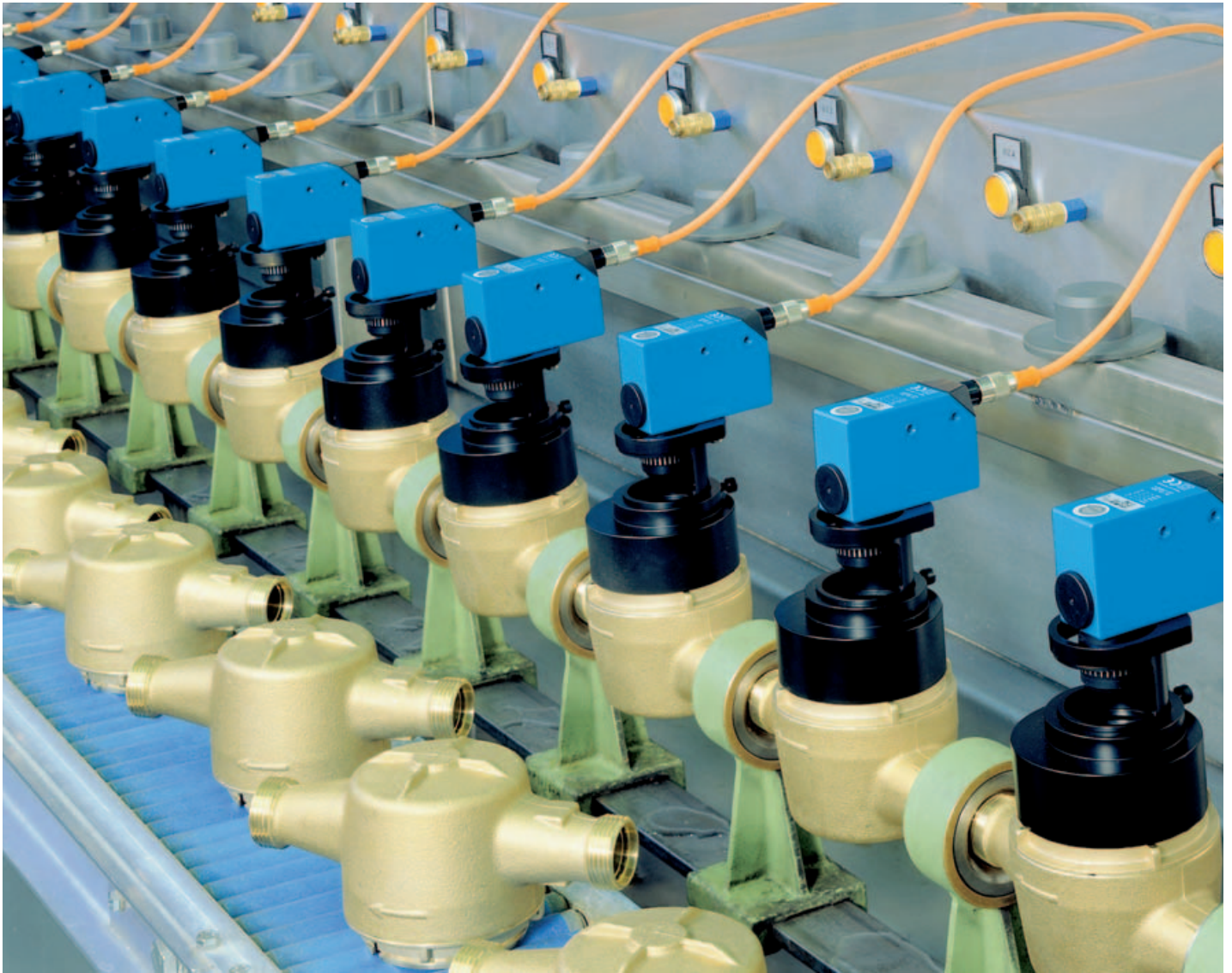
▲ KT contrast scanner in water meter manufacture Easy parameter management through integration into CAN network
