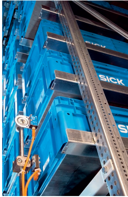
▼ ► Precise positioning of stacker cranes using the holes in the carriers.
