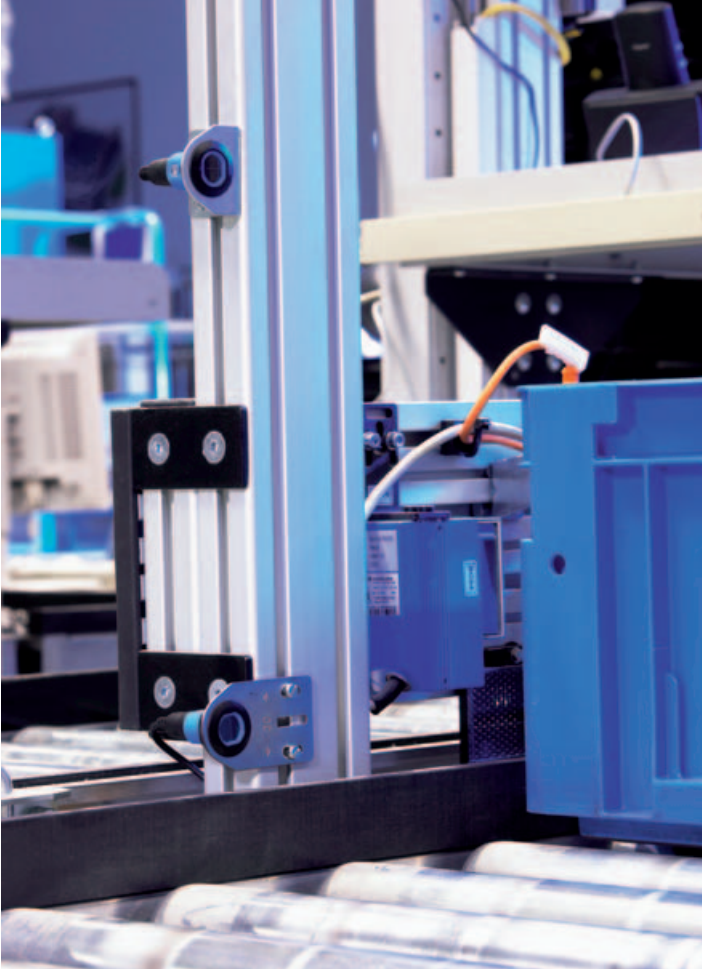
▼ Height control with an MHL 15 photoelectric reflex switch , for sorting containers on a conveyor belt.
