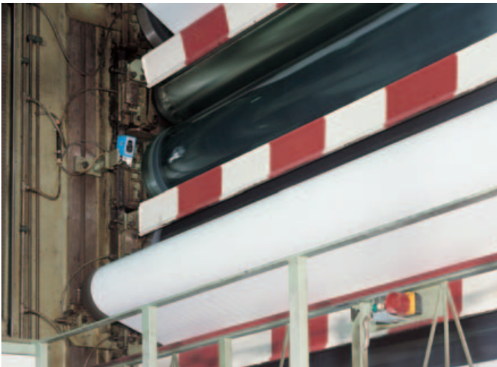
▶ A WS/WE45 through-beam photoelectric switch monitors tear-off on a paper web.
