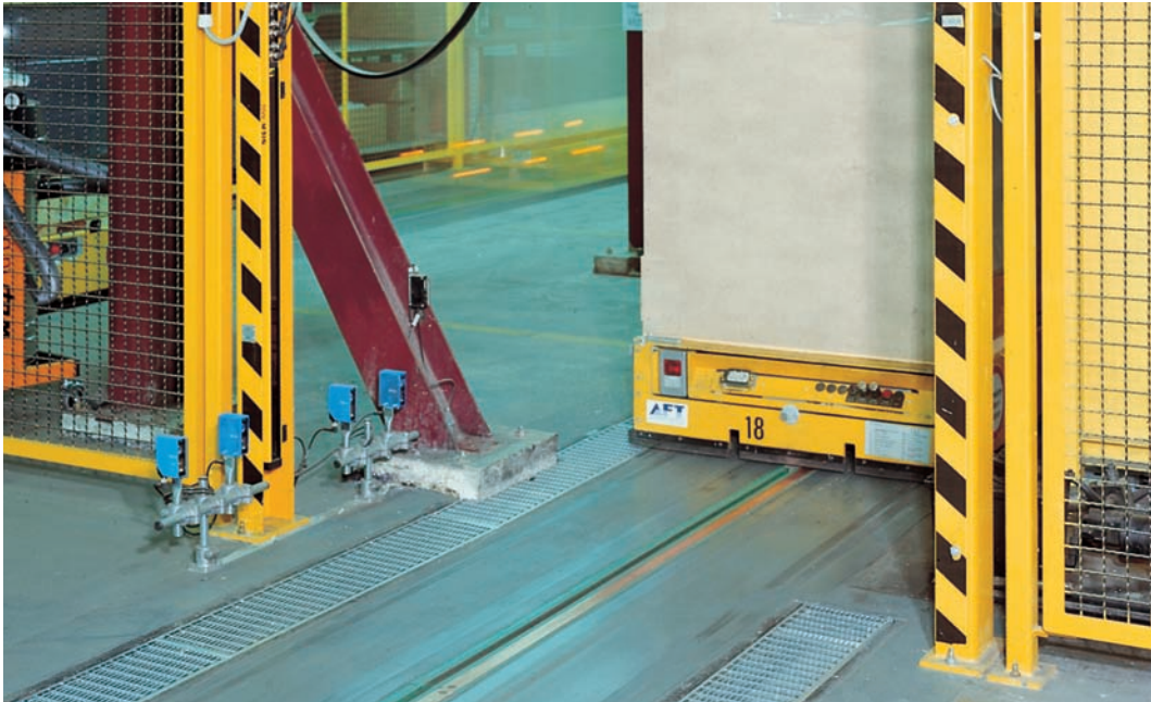
◀ Used as muting sensors, WT 24-2 photoelectric proximity switches signal the entry of an industrial truck into a protected zone and clock the multibeam photoelectric safety switch.
