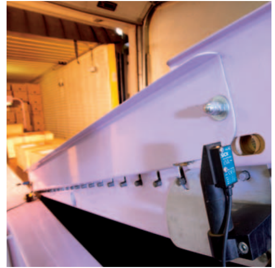
▲ W 9-2 in warehousing and conveying technology; universally installed, secure, compact.
