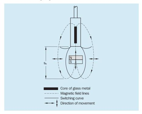
Case 2: The sensor responds if the magnet approaches the switching curve laterally. If the sensor leaves the switching curve, the sensor switches back again. This principle is largely used for magnetic cylinder sensors.
