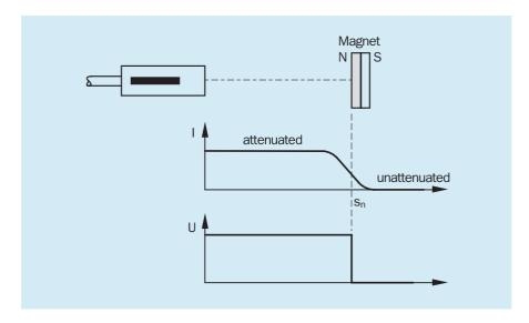
Permanent magnets are usually used to trigger magnetic proximity sensors. They comprise magnetically hard substances – steel alloyed with other metals such as aluminium, cobalt and nickel. Magnetically hard ferrite with similar properties can be also be produced from sintered compounds containing iron oxide and other metal oxides.
