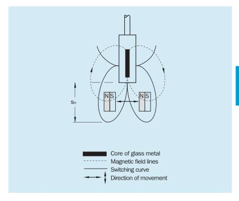
Case 4: In this case, the magnet passes through two switching curves. The magnetic field reverses at the boundary of these curves and two switching points are produced. The detection of this interruption again depends on the actuating speed and the radial distance relative to the sensor axis.
