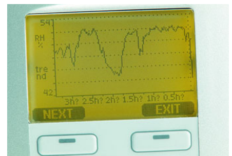
With the help of the display, the user is able to trace measurement trends back for up to a year.
