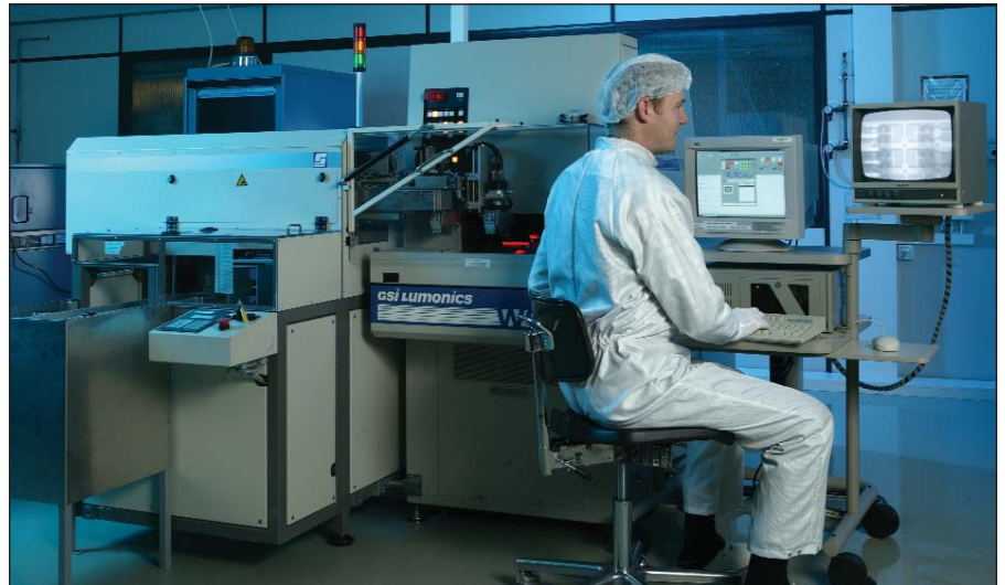
Fig. 6: Producing temperature sensors under clean-room conditions
