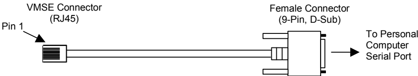
Figure 6-8. Cable for Serial Monitor/Load of VMSE
