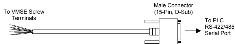
Figure 6-12. VMSE Screw Terminals to 15-Pin D-Sub PLC Serial Port
