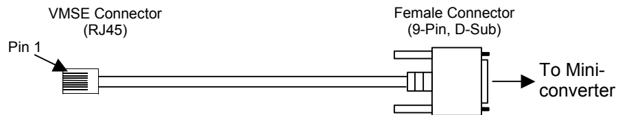
Figure 6-6. VMSE RJ45 Serial to RS232/485 Miniconverter
