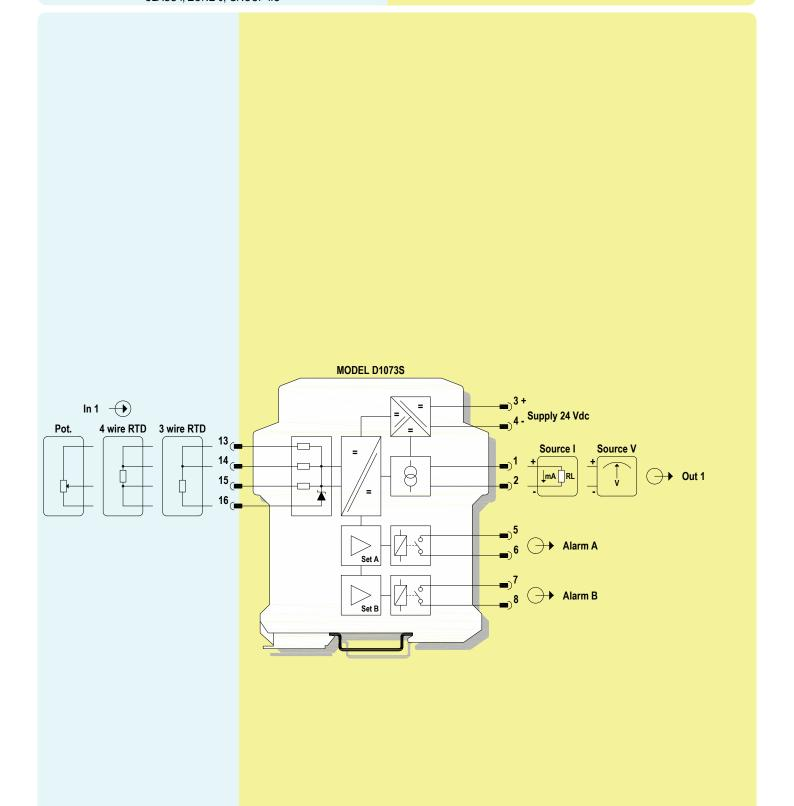
For SIL applications, alarm contacts must be used in series with equal configuration. Relay contact shown in de-energized position
