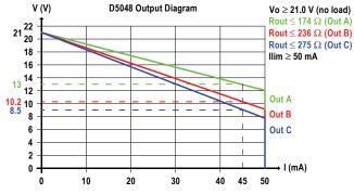
**Short circuit current:** ≥ 50 mA (55 mA typical). **Response time:** 75 ms.
