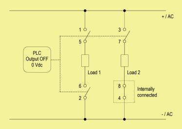
Contacts 1-5 and 2-6: Closing of contacts can be used for monitoring
