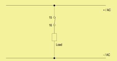
Contacts 15-16: Voltage free contact for Line and Load Fault detection.
