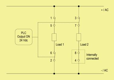
Contacts 1-5 and 2-6: SIL 3 Function is met when contacts are in open state.
