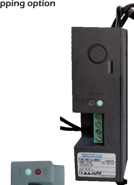
The green led in ready and ok state and the red led in the failure situation.
