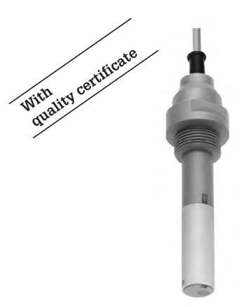
The compact conductivity measuring cells have been designed especially for measurement in high conductivities. The measuring cells with a Pt 100 temperature sensor are used together with conductivity measuring instruments of the Mycom, Liquisys and MyPro families, equipped with the automatic temperature compensation.
