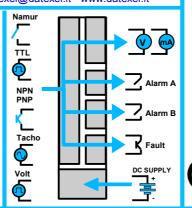
Configurable by Dip-Switch or PC, Transistor or Relay Outputs DAT 4540
