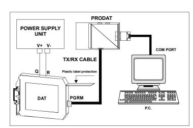
Warning: during these operations the device must always be powered and the TX/RX cable always connected. For information about DATESOFT refer to the software's user guide.
