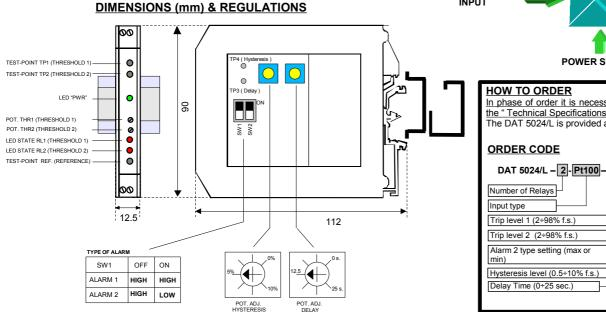
uded in the The DAT 5024/L device is suitable for fitting to DIN rails in the vertical e terminals position. For optimum operation and long life follow these instructions:
