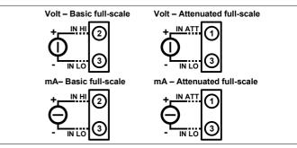
$(^{\star\star})$  Note: if the input signal is isolated from the power supply the terminal 3 (IN LO) must be connected to the terminal 4 (COM).
